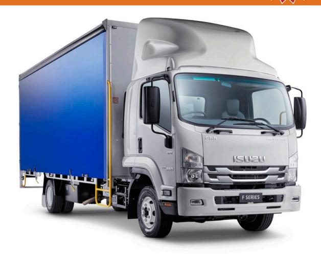
10 pallet (nominal) curtainside body / Easy glide curtains with quick release "Lightning" latches / Lightweight side gates /
